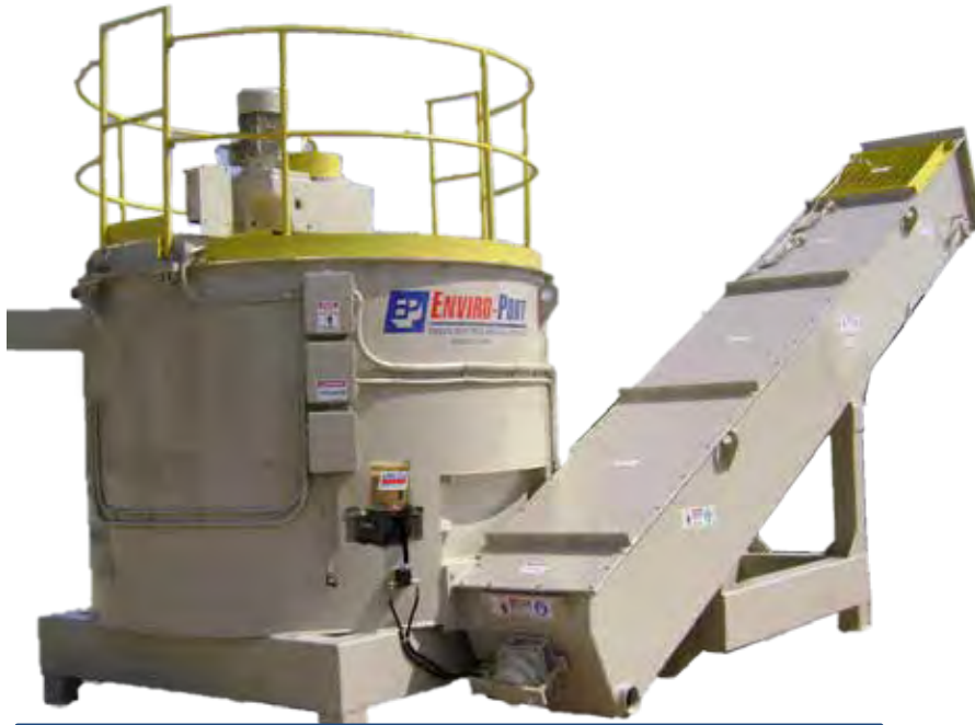
B13-2000 Basic Separation Unit Dry Weight 15,400lbs, Full Load Weight 35,400lbs
